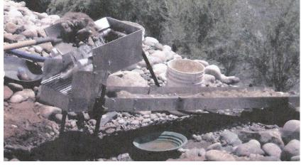
observed that the first stage in the hopper box retains the greater amount of gold and the other sections in line decreasing until the final section contains almost nothing. Since the first stage contains the most gold and also the least amount of sand, it should be "harvested" regularly and the next stages can be run much longer with the final stage cleaned at the end of the day. Also checking this stage will tell if the gravel that is being processed has any gold or other value.
